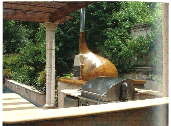
Wood-fired ovens can be built in various sizes and forms. A round oven like this one heats up fairly quickly and evenly, which makes it ideally suited for cooking pizza. Courtesy of Fogazzo Wood Fired Ovens and Barbeques
